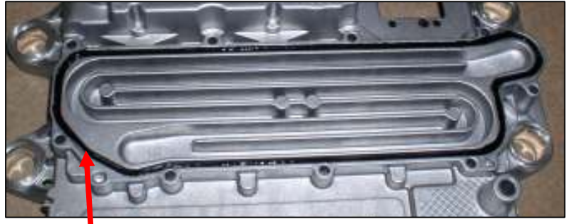
Bottom section with channel filled with sealant
